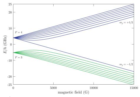
Figure 4: Cesium  $6^2S_{1/2}$  (ground) level hyperfine structure in an external magnetic field. The levels are grouped according to the value of F in the low-field (anomalous Zeeman) regime and  $m_J$  in the strong-field (hyperfine Paschen-Back) regime.
