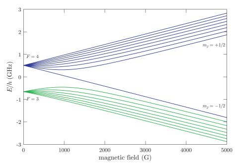
Figure 5: Cesium  $6^2P_{1/2}$  (D<sub>1</sub> excited) level hyperfine structure in an external magnetic field. The levels are grouped according to the value of F in the low-field (anomalous Zeeman) regime and  $m_J$  in the strong-field (hyperfine Paschen-Back) regime.
