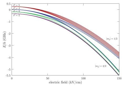
Figure 7: Cesium  $6^2\mathrm{P}_{3/2}$  (D<sub>2</sub> excited) level hyperfine structure in a constant, external electric field. The levels are grouped according to the value of F in the low-field (anomalous Zeeman) regime and  $|m_J|$  in the strong-field ("electric" hyperfine Paschen-Back) regime. Levels with the same values of F and  $|m_F|$  (for a weak field) are degenerate.
