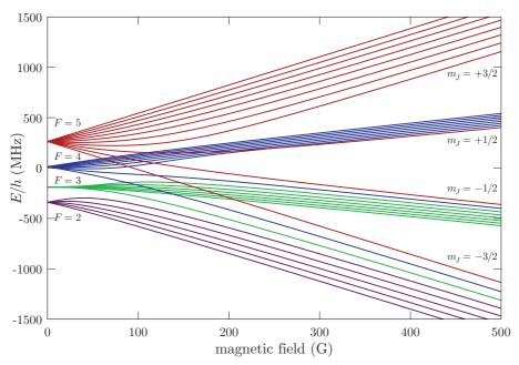
Figure 6: Cesium  $6^2P_{3/2}$  (D<sub>2</sub> excited) level hyperfine structure in an external magnetic field. The levels are grouped according to the value of F in the low-field (anomalous Zeeman) regime and  $m_J$  in the strong-field (hyperfine Paschen-Back) regime.
