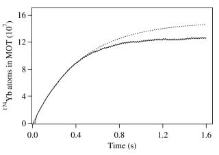
**Fig. 6.** Nonlinear losses. The number of  $^{174}$ Yb atoms in the trap (solid line) increases exponentially at first, but saturates at a lower value due to the  $N^2$  loss term in equation (1). The dotted line is the extrapolated exponential curve.
