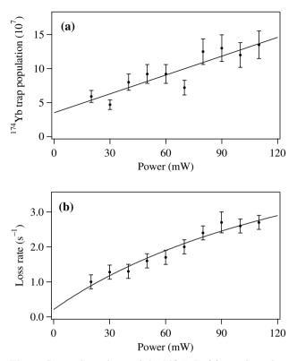
Fig. 5. Power dependence of the MOT. In (a), we show that the number of trapped  $^{174}$ Yb atoms increases linearly with trapping power. In (b), we study the loss rate as a function of power. The solid line is a fit to equation (2) in the text and allows us to separate the loss rates due to collisions and branching into metastable levels.
