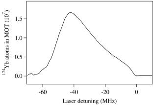
Fig. 3. Number of trapped atoms vs. detuning. The number of  $^{174}$ Yb atoms in the MOT is shown as the detuning of the laser is varied slowly from -60 MHz  $(-2\Gamma)$  to 0. The magnetic field gradient at the trap center was 75 G/cm. The number of atoms shows a peak at -42 MHz or  $-1.5\Gamma$ . Other isotopes show identical behavior.
