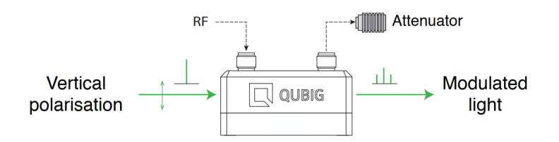
The use of a long coaxial cable between the EOM and the RF attenuator is recommended to avoid heating for high RF power.
